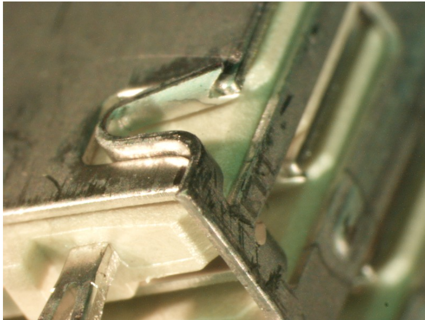
Figure 6. Formed Interconnection Feature at Bottom Rear of METRAL® 1000 Receptacle – 20X
