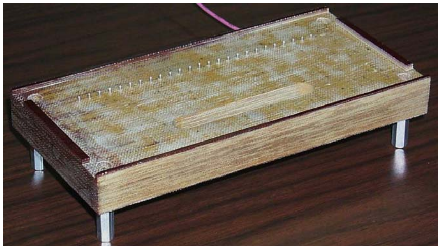
Figure 3. Fixture for Low Level Compliant Pin Resistance Measurement
