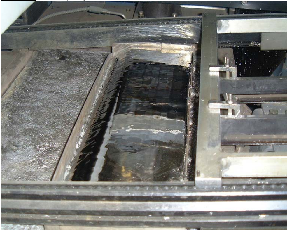
Picture 5 : PCB on the wave
