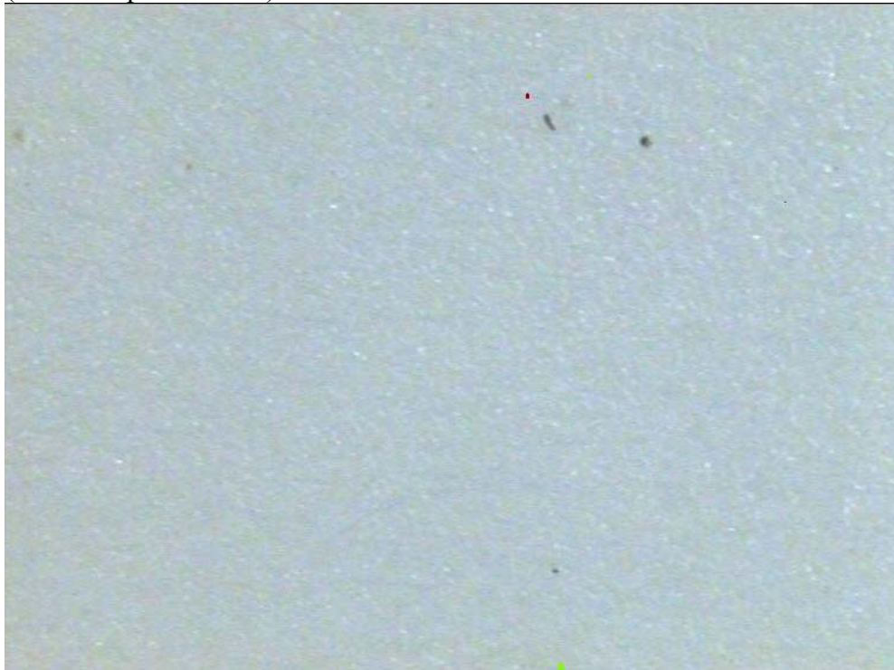
Picture 22 : female right angle DIN in PBT Valox 420SEO at 265°C with Kapton protection (correct aspect surface)
