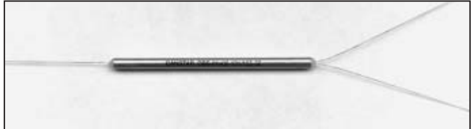
BS - type, 250 µm coated fiber leads for most compact size.
