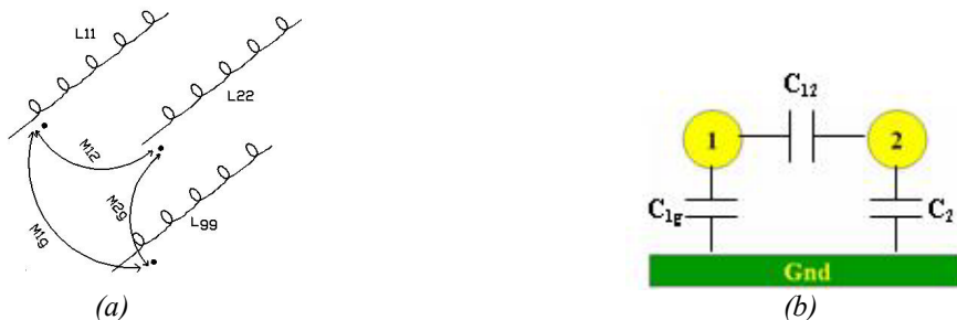
Figure 2: (a) Partial Self and Mutual Inductances Associated With Each Conductor in Figure 1(a). (b) Equivalent Capacitance per Unit Length Between Each Conductor in Figure 1(a).
