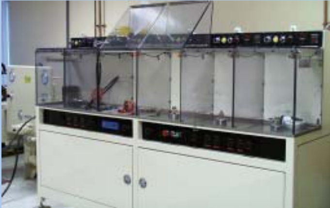
Hydraulic Test Machine, conducts life cycle testing of tool heads by applying pressure ranges of 10 000 lb/in 2 (68.9 MPa) to 27 000 lb/in 2 (186.2 MPa). This type of testing is done to evaluate the life of existing tools and new tools.
