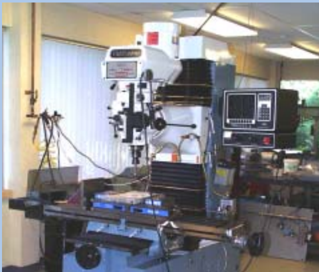
Model Shop - CAM (Computer Assisted Machining). Prototype made from Pro-Engineer solid model electronically transferred to the equipment.
