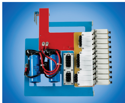
Power distribution unit for a wireless base station distributes power to a bank of circuit breakers
